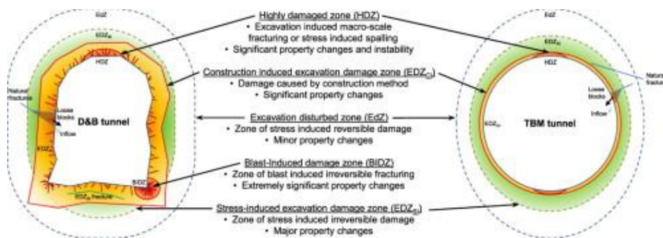
Fig. 2 Excavation damage terminology in hard crystalline rock (Siren et al., 2015)
